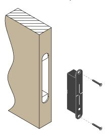
3e. For the door side unit, drill a wiring channel to the electrified device to be powered.
