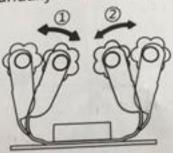
When the installation is completed, use 3kgf force to pull the handlebar toward the arrow direction. If the tire does not come out, the installation is completed. If it does, readjust the size of C clamp until the tire does not come out.
