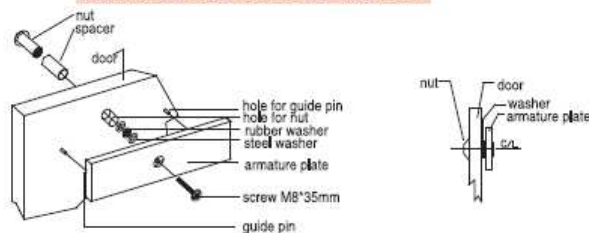
Armature Plate Mounts To The Door
