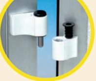
Adjustment of closing pressure Just rotate the lower bushing to the three different settings (-0.5;0;+0.5 mm)
